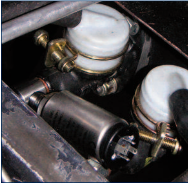
1500 Series pressure sensor being used to test hydraulic brake performance.
